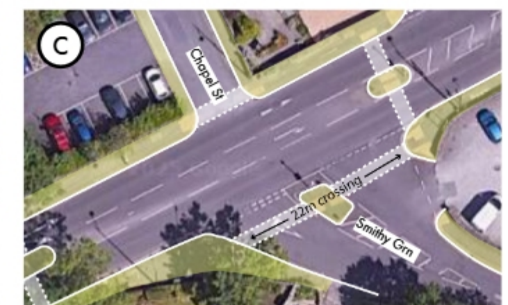
Intersection design encourages quick vehicular speeds around corners, while providing minimum protection for pedestrians crossing.
