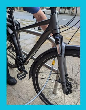
2. Feed one end of the cable, through the whole on the other end, so the cable hugs the tire. 3. Loop the end of the cable through the back tire and around to the frame.
