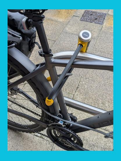
4. Place the D Lock around the frame, ensuring it also goes through the loop at the end of the cable. Ensure everything is secured to the frame.
