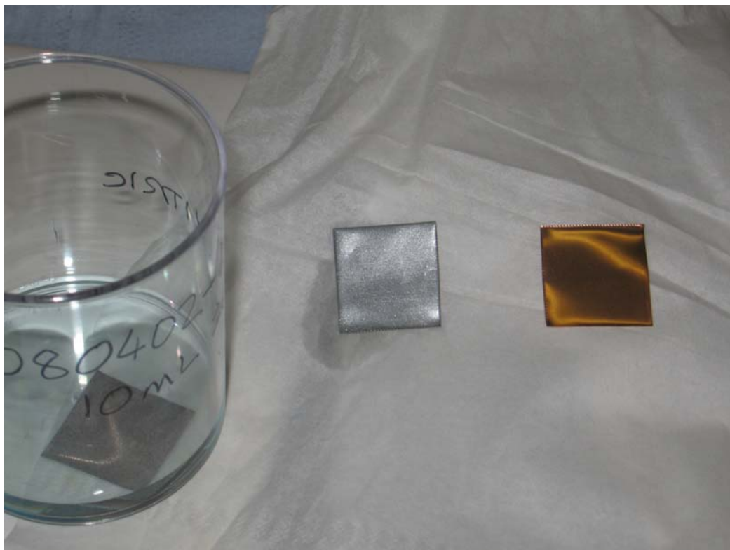
Figure 1 From the left: a copper coupon immersed in solution; copper coupon with mercury deposited on surface; unused copper coupon for comparison.
