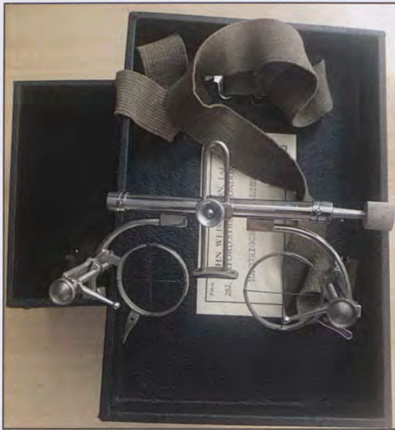
Figure 4. MacGrigor Localiser with its box
