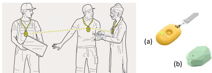
Fig. 1: (a) proximity wearable device worn with lanyard - can also be worn in a front pocket without lanyard; (b) static beacon (adapted from https://estimote.com/ )
