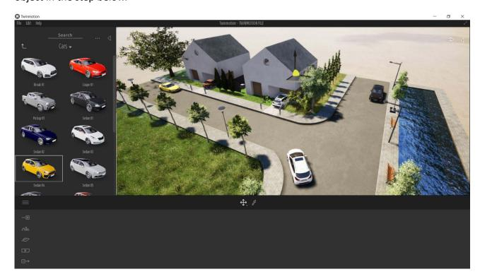
• To **rotate** a car or any objects in Twinmotion, again click on the object and then click and drag the yellow arc in the xyz axes as below
