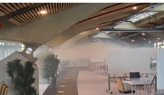
All vents closed: entrainment to radiator plumes. Gravity currents. Strategy needed to avoid lock-up layer and thermal discomfort.
