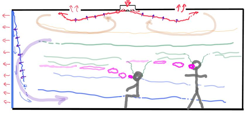
Net effect: establishment of a **strong** internal stratification and very low effective ventilation rate.
