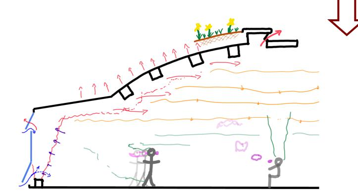
All vents opened: most incoming air into the plume. Some causing cold drafts at floor level. Thermal discomfort. Some ventilation by air entrainment into the plume. Less strong internal stratification.
