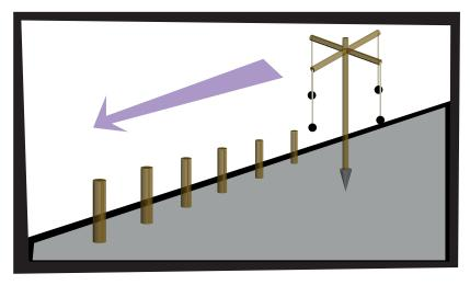
9. To check the accuracy of the posts, take the groma to the end of the line and look down the line. Adjust if necessary.
