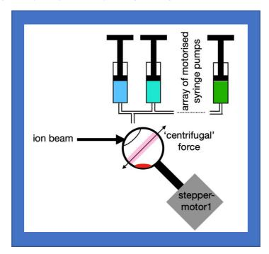
This sample holder is a 3D printed in polypropylene spherical shaped open topped vessel with a stem. This stem allowed the attachment of an electric motor to the sample chamber.
