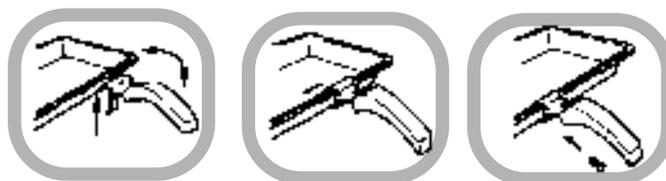
The grill pan handle is detachable from the pan, to facilitate cleaning and storage. The handle can be either detachable from or fixed to the pan. For a fixed handle remove the screw and washers from the grill pan bracket, tilt the handle over the recess adjacent to the bracket.
