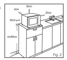
WARNING: Do not install oven over a hob or other heat-producing appliance. If installed near or over a heat source, the oven could be damaged and the warranty will be invalidated.
