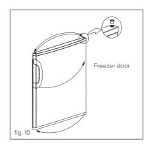
8. Rotate the central hinge 180°.
