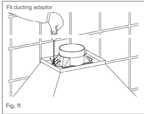
**IMPORTANT SAFETY WARNING:** ONLY USE THE SCREWS PROVIDED WITH THE EXTRACTOR TO MOUNT THE DUCTING ADAPTOR. THE USE OF LONGER SCREWS MAY CAUSE DAMAGE TO THE INTERNAL WIRING WHICH WILL NOT BE COVERED BY THE GUARANTEE.
