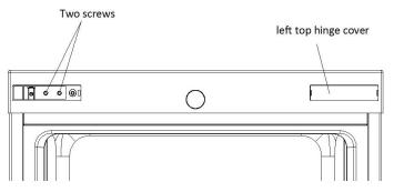
8) Install the top-hinge. set the top door right position, fix the top-hinge and the cover.
