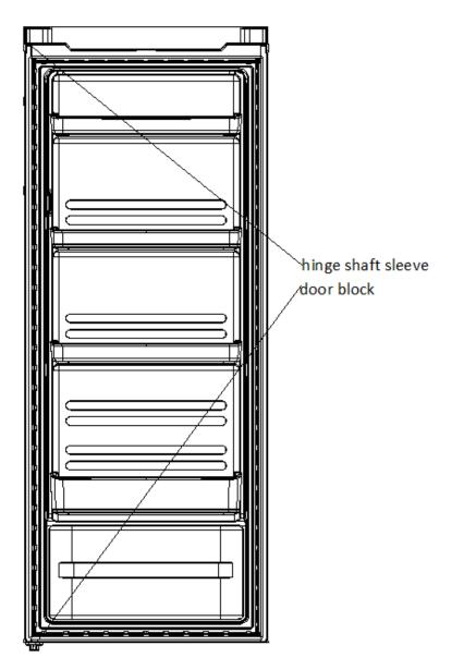
4) Disassemble the screws fixed the bottom hinge assembly with cross slot screwdriver and remove the adjustable foot
