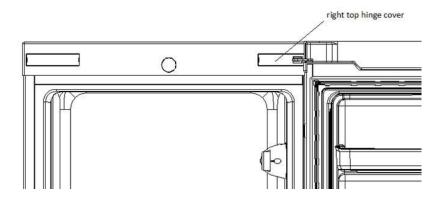
2) Remove the screws fixed the top-hinge with cross-slot screwdriver.
