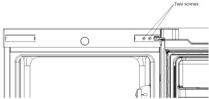
3) Remove the hinge shaft sleeve and the door block to the other side.
