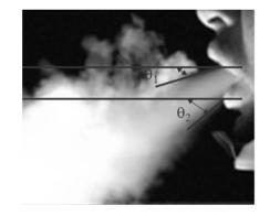
The exhaled droplets are modelled as particles, which are injected with the exhalation flow and interact with the room air
