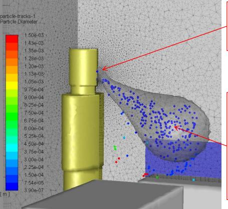
The flows of room air and exhaled breath are calculated on a mesh which is fitted to the geometry
