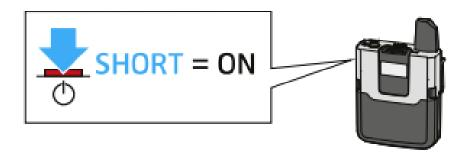
The home screen appears on the display panel (see "Displays on the display panel of the SL Bodypack DW"). The status LED indicates the current status of the receiver (see "Meaning of the status LED on the bodypack transmitter"). The radio link to the last paired receiver is established automatically as soon as the receiver is switched on.
