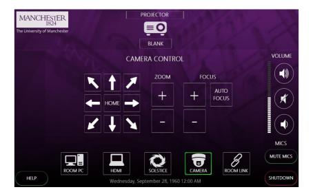
The arrow buttons can be used to adjust the pan and tilt of the camera and the HOME button to reset its position. + and – buttons are available to adjust the zoom and focus and auto focus can also be set.
