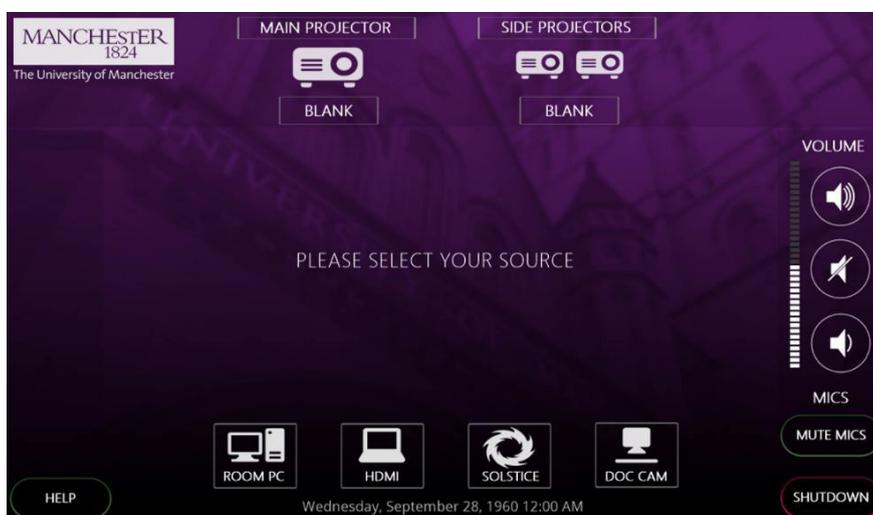
There are four available sources, ROOM PC, HDMI, SOLSTICE and DOC CAM. The first time a source is selected the user will be prompted to select a projector on which to view it. Pressing the desired projector will switch the projector on, this will usually be MAIN PROJECTOR. The confidence monitors will also power on and duplicate the content on the main, or central projector. Repeat the process for the desired source for the SIDE PROJECTORS.
