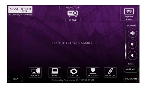
There are five available sources, ROOM PC, HDMI, SOLSTICE, DOC CAM and ROOM Link. Pressing any of these will power up the projector and additional screens, displaying the selected source, (on initial start up the additional screens will mirror the projector). The currently displayed source can be changed at any time in the same manner.
