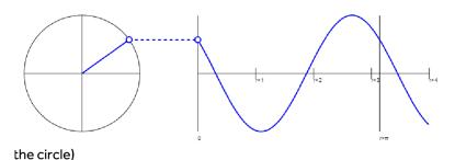
A sinewave is defined as the projection of a point moving at a uniform speed around a circle, onto an axis. (imagine the point rotating around
