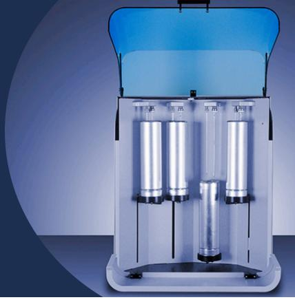
Quadrasorb EVO Surface Area & Pore Size Analyser provides fast and accurate B.E.T. (Brunauer, Emmett and Teller) surface area measurements, by characterising the porous structure of materials, and providing the specific surface area (SSA), specific porous volume (SPV), and pore size distribution (PSD) of a sample.
