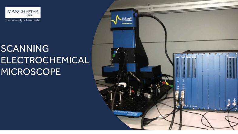
Scanning electrochemical microscopy measures the local electrochemical behaviour at a liquid-solid interface. Typically, a solid sample is used and forms the counter electrode. This sample is immersed in electrolyte and a ultramicrocapillary containing the working electrode is scanned across the surface.
