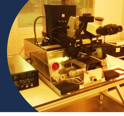
Conventional optical lithography uses an etched chrome photomask to transfer the required device design into a photo-resist coated substrate. The NGI uses a Karl Suss MJB4 mask aligner for this purpose.
