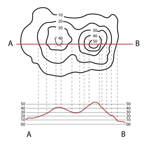
In the example above, the contour lines show the different levels of the hill on the layout (10,20,30,40,50). A cross section line AB is drawn. The points of known levels are pulled to the cross section profile below. Then every point was assigned to its value in which the 50m points are at the top of the hill, whereas the 10m points are at the bottom of the hill.
