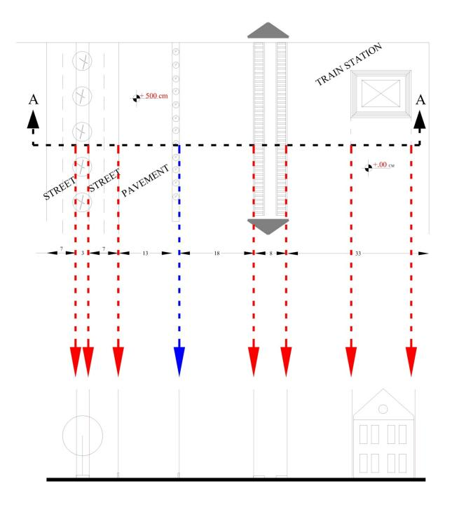
Now we need to identify the height of the objects. The first thing in this stage is drawing the correct land line with the correct levels. The blue arrow above shows the point where the land level changes from +-0.00cm to +500cm. As shown on the figure below, measure 500cm (i.e. 5cm in the 1/100 scale if you are drawing by hand) on this vertical line and draw a point. From this point draw a horizontal line heading left. This is the +500cm ground level.
