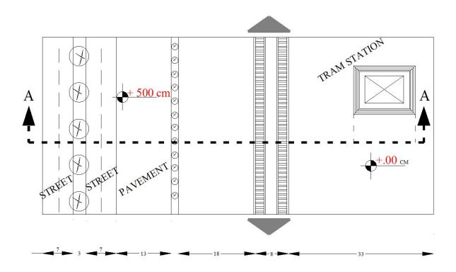
The land topography (the existence of two levels) encourages us to do a cross section to start analysis. The first thing to do is drawing the land profile. You can do this by hand or by CAD. First, draw a strait land line .All the objects on the layout (the borders of the building, the tram lines, the edge of the upper level, the street...etc ) should be pulled down to the land line. They should appear as vertical lines on the cross section.
