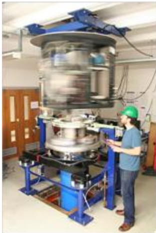
Rotating millikelvin cryostat that allows visualization of vortex lines in superfluid
