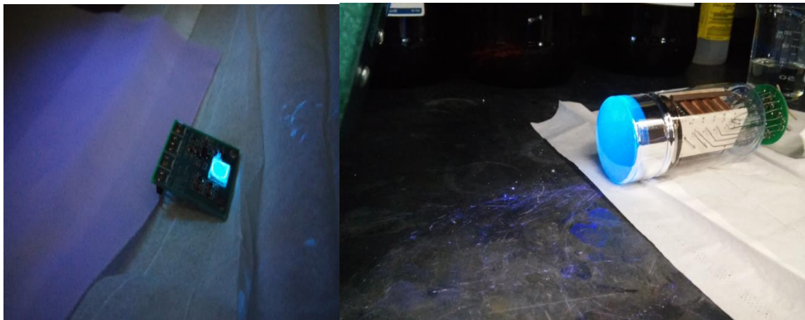
Silicon photomultiplier and cryogenic photomultiplier covered in a blue-emitting wavelength-shifter under UV lamp light.
