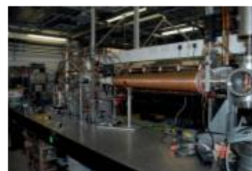
An atom cooling and trapping set-up, showing the source chamber (right), Zeeman slower (centre) and trapping chamber (left).
