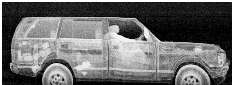
Figure 1. X-ray backscatter image of a car with contraband hidden within the body panels. These areas show up as brighter regions of the x-ray image. No detailed material information is currently possible. Obtaining detailed material information is the aim of this work.
