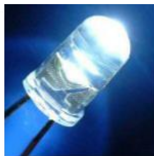
An LED based on InGaInGaN quantum wells.
