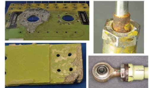
Top Image: Products manufactured by processes which depend on Hexavalent chrome technology at end of service life. (Image: Goodrich Actuation Systems Ltd)
