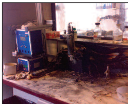
Fire at a weekend when an experiment was left unattended. Fire detection and prompt action prevented the outcome being much worse.
