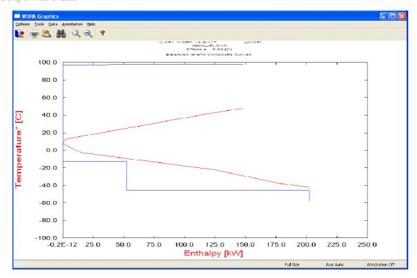
**WORK** can optimise the composition of mixed refrigerants to minimise shaftwork requirements. This is achieved by optimising the composition of the refrigerant to match the cooling profile.
