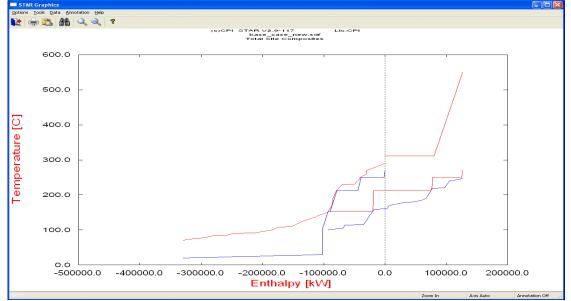
Site composite curves illustrating heat recovery between processes via the site steam system
