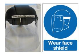
All laboratory work with UV sources necessitates the use of full face shield with visor (to protect the neck and face area fully) and gloves to protect the hands and wrists, to the <u>BS EN</u> <u>170</u> standard.
