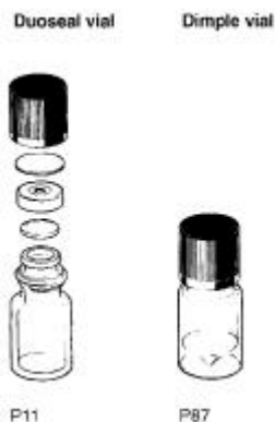
Fig 3. Schematic of the duoseal and dimple vials.
