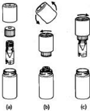
Fig 5. Schematic of Amersham Biosciences' microvial (type P15).
