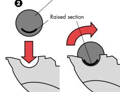
With raised section on end of brush bar orientated as shown, locate brush bar in slot and rotate end cap towards back of machine until it comes to a stop.
