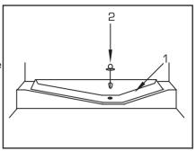
If, at any time, the defrost water does not drain from the collection channel, check that no food particles have blocked the drain tube. The drain tube can be cleared by pushing the special plastic plunger provided down the drain tube.
