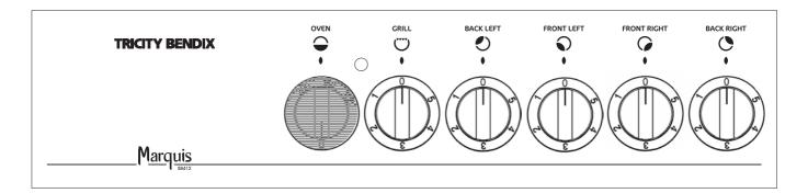
To operate the oven turn the oven control to the required temperature.
